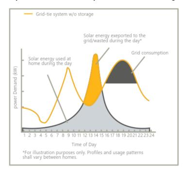
By storing the surplus PV generation into battery storage unit, it can maximize PV generation and reduce electricity bill.
