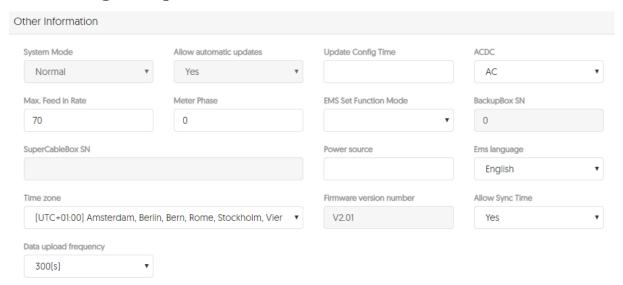
Installer can set the max feed-in rate on the other information interface of the "System Setup" page.
