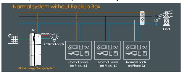
If the grid fails, the energy storage system will only provide power to the critical loads which are connected to the backup port.
