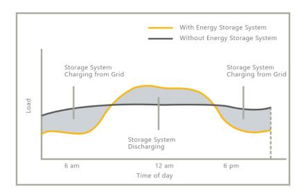
Especially when the electricity tariff is different in one day, you can set battery grid charging time on EMS LCD, on AlphaCloud monitoring portal or through AlphaESS App.
