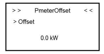
The default PmeterOffset of the system is 0, that means the peak shaving function is off.
