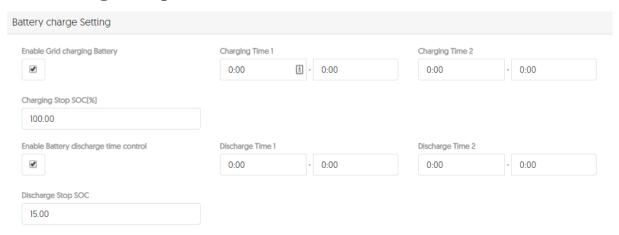
End user can set the grid charging time and battery discharging time on the portal or through AlphaESS App.
