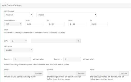
Click AUX Contact Channel to choose AUX 1 or AUX 2. Two devices can be controlled.
