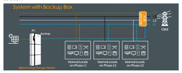
If the grid fails, the energy storage system will provide power to all loads.
